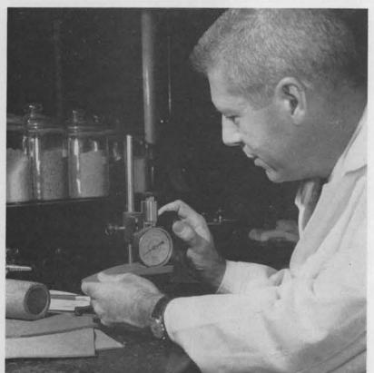
TESTING HARDNESS of rubber is George Dykes (1625). This is one of the many tests new materials must undergo in the development of experimental weapon components at Sandia Corporation.
